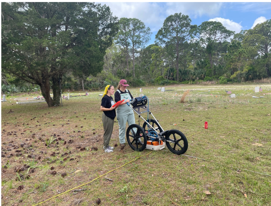
Interns Maria Fortune and Lydia Hawk conducting a GPR survey at Saints and Sinners Cemetery in Oak Hill.
